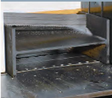
The saw head swings up to 60° both ways with programmable go-to settings for versatile production cutting while reducing material handling time.
