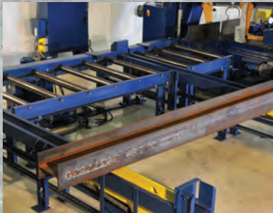
Cross transfer feeding to roller conveyors
